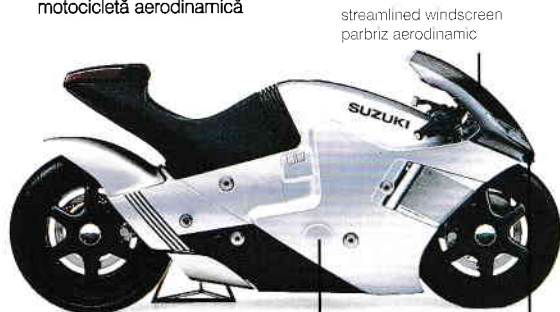
fairing (streamlined bodywork) invelis aerodinamic
